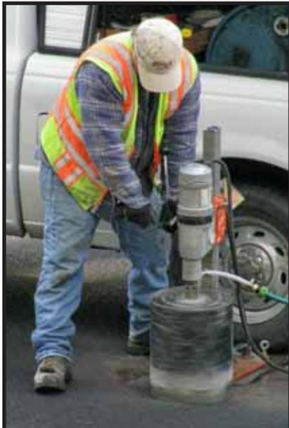
*Geotech test technician cores a pavement sample from Kala Point Drive on March 31st. The sample was then laboratory analyzed for density & material make-up.*
